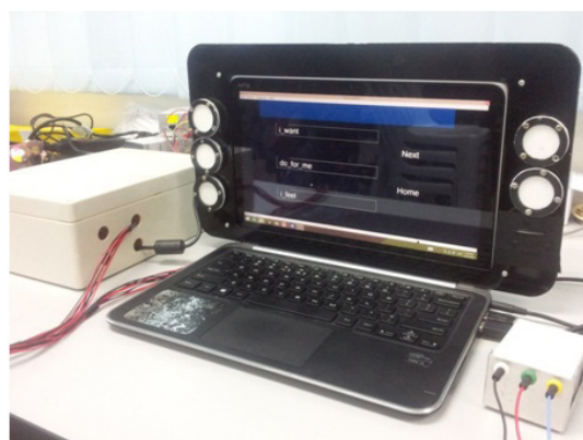
Figure 1. BCI systems. Photographs showing BCI systems featuring LCD (left) and LED stimulators (right). The units on the right of both photos are the EEG acquisition module.
