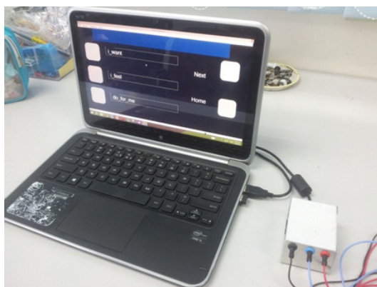
Figure 1. BCI systems. Photographs showing BCI systems featuring LCD (left) and LED stimulators (right). The units on the right of both photos are the EEG acquisition module.
